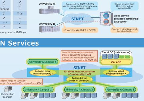
• SINET side: Automatically recognizes VLAN-IDs at SINET nodes and automatically connects between multiple points.
