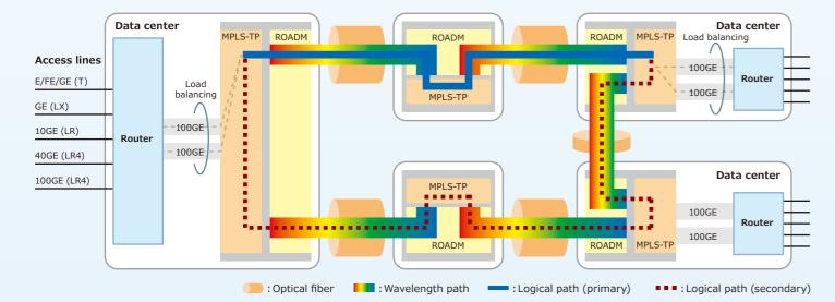
Routers set logical systems (LS) for each group of services. Individual LSs are connected by VLAN connections.
